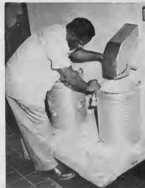
CUBES ARE automatically fed from storage hopper to the water coolers with the help of gravity. Filling coolers for the field is C. C. Barkel. CUBANAN TA wordé automaticamente trasladi for di storage hopper pa e contenedoran cu ayudo di gravedad. Yena pa e contenedoran pa field ta C. C. Barkel.
